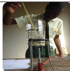
Fig. 5.5: Determining the upper fixed point on a thermometer
